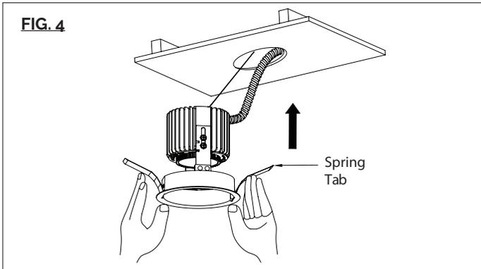
4. Fold trim assembly mounting springs inward and insert trim assembly into ceiling cutout. Be sure once installed, trim assembly is flush and secure (See **FIG. 4**).
