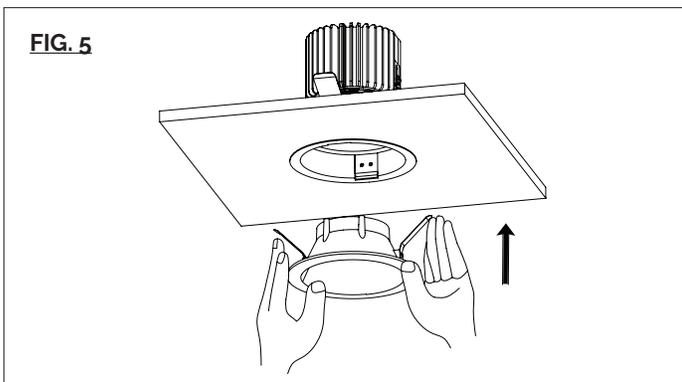
5. Raise trim into trim assembly. Be sure trim springs go into slots in assembly. Raise trim flush with ceiling surface (See **FIG. 5 & 6**).
