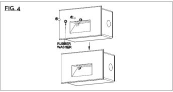
Place all wiring and connectors back in junction box and install the fixture.
