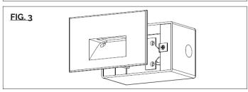
Connect the fixture wires to the junction box wires as follows: Black fixture wire to black (Hot) J-BOX wire, white fixture wire to white (Neutral J-box wire, and green fixture wire to Ground. (See Fig.3).
