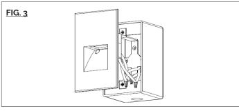
Connect the fixture wires to the junction box wires as follows: Black fixture wire to black (Hot) J-BOX wire, white fixture wire to white (Neutral) J-box wire, and green fixture wire to Ground. (See Fig.3)
