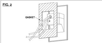
3 Insert gasket onto the back of the fixture (Fig.2).
