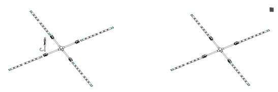
24VDC Basics Flex X & Y Connector can be used for power feeding by using low voltage wiring box (A2L36-WT). Make sure that polarity is correct.
