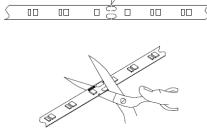
Mount Tape Light: Clean surface before mounting. Peel off 3M adhesive backing cover off as strip is installed, pressing firmly to mounting surface in increments.
