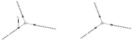
24VDC Basics Flex X Connector (A2L39-WT) - the wire insulation jacket shall be stripped, Make sure polarity matches between tapes.
